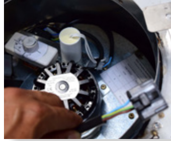
Pull the cable to the top of the termination and attach to the connection block as shown below. Please ensure that the leads do not touch the motor in any way (cable tie if necessary).
