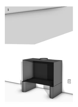
Install the LFS800 Console in the desired location. The console should be a min. 50mm off the wall behind. Allow for the power supply to the fireplace.
