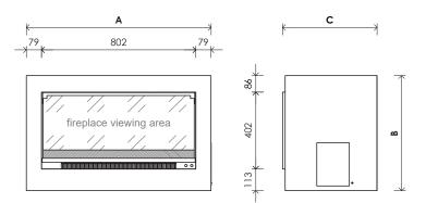
Install in accordance with AS/NZS3000 and the Escea LE Series Install Manual.
