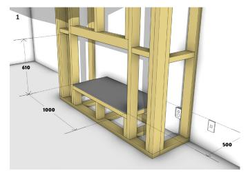
Build the chimney framework with consideration to the minimum cavity opening requirements (1000mm W x 610mm H x 500mm D). Ensure a continuous base for the fireplace.
