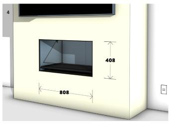
Attach wall linings to the framework and fireplace, maintaining a 3mm gap from the fireplace trim. Follow the provided wall lining cutout dimensions above. Complete the project by adding additional finishes or fixtures.
