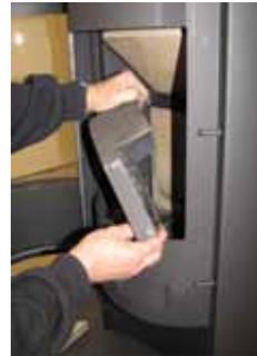
4. Lift the bottom baffle plate again and tip the other brick panel out.
