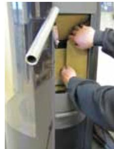
5. Lift the bottom baffle plate free of the tertiary combustion air box and remove it.
