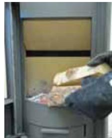
The stove door should normally be opened gently the first 2-3 cm, then you should wait until the pressure has equalised before opening the door all the way. This technique will prevent smoke from getting out, particularly when there is a poor draught.
