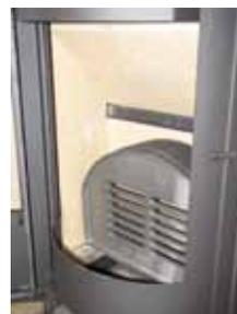
2. With one hand, lift the bottom baffle plate. With the other hand, lift the brick panel up a few centimetres. This is best done with a slotted screwdriver or similar. Once the brick has been lifted, tip the diaphragm back into place, so the brick panel is now released and can be lifted out.
