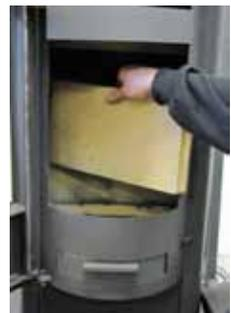
6. If necessary, the rear brick can now be removed.
