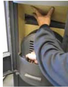
3. Once the first brick panel has been removed from the stove, the diaphragm can be lifted and removed.
