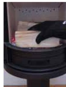
The stove door must be opened gently the first 2 - 3 centimetres, then you should wait until the pressure has equalised before opening the door all the way. This technique will prevent smoke from getting out, particularly when there is a poor draught.
