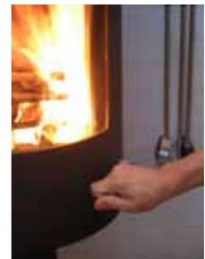
5. If the condition in step 4 is met, place max. 2 pieces of wood with a total weight of 1.5-2 kg and a length of 25-30 cm over the embers in a single layer, with a distance of approximately 1 cm.
