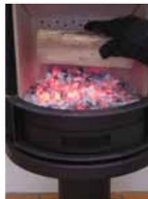
6. Open the air supply to maximum, and close the door. The fresh wood will be lit within 2-3 minutes.
