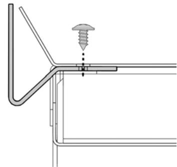
To attach the Inset Fascia a magnet bracket must be fixed to the firebox. This bracket slides in to sit flush with the underside of the top firebox panel. To secure it in place screw the provided pozi-drive screws into the four holes, positioned behind the 45 degree flange at the top edge of the firebox.
