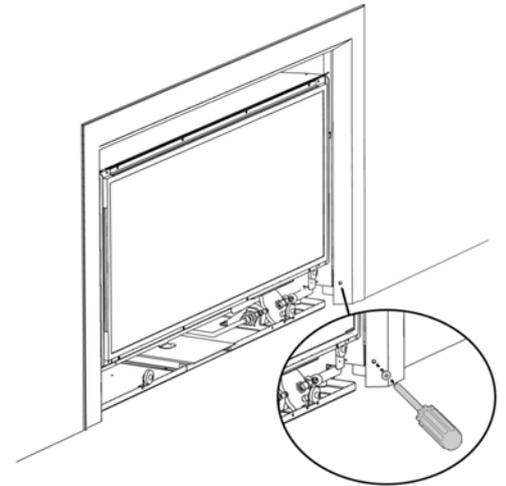
**Step 5:** Attach the inner fascia brackets to the Inner Fascia as per the instruction page supplied with the fascia. Hang the top edge of the Inner Fascia (smaller one) from the lip that extends at 45 degrees from the top of the firebox. This fascia is attached to the fire at its base by two screws. Leave the screws loose enough to be able to adjust the Inner Fascia.
