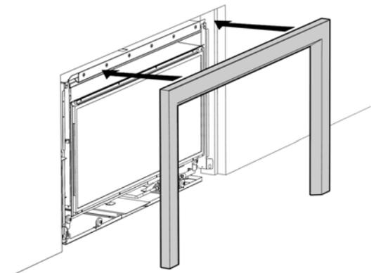
**Step 4:** Fit the two screws at the base of each side of this fascia. The heater may have to be adjusted in or out of the cavity to ensure fascia fits correctly.
