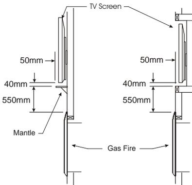
When building a recess the flueing must be considered. Shown right is the minimum distances possible when offsetting the flue to allow for a recess above using Escea's standard flue kit.
