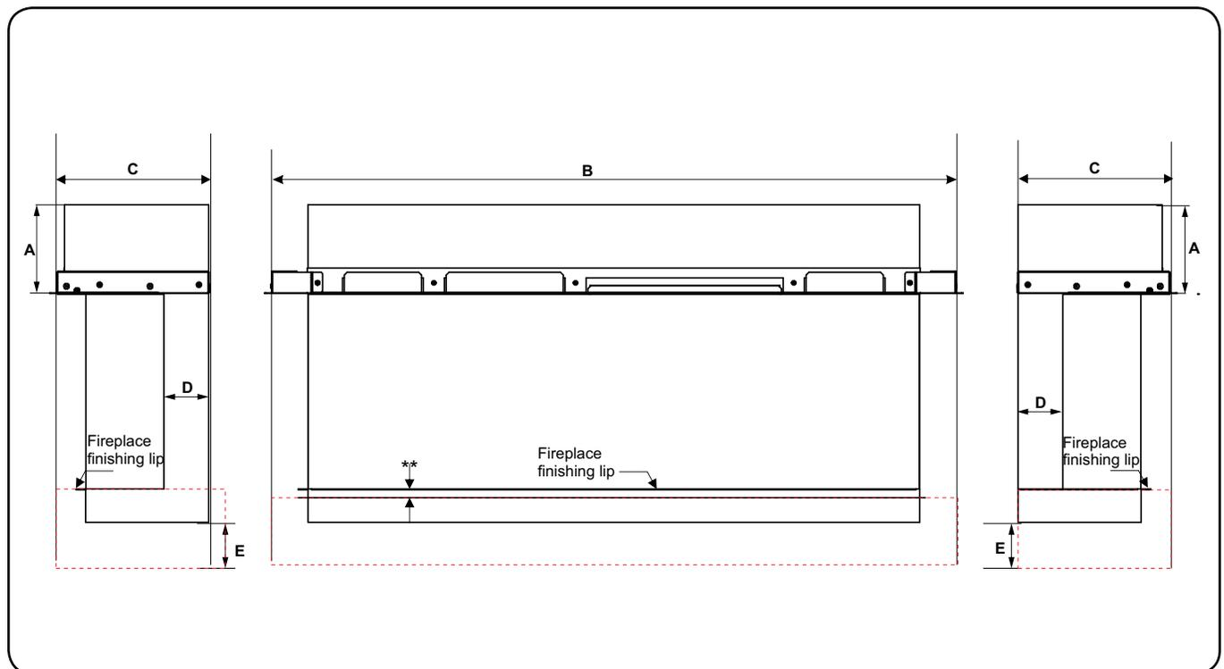
**Important:** The appliance must be mounted to the wall prior to framing. The wall in behind the appliance should be drywalled prior to installing the appliance for ease of finishing.
