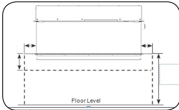
3. The lower enclosure can locate over or under the lower flange on the product, see Diagram below.
