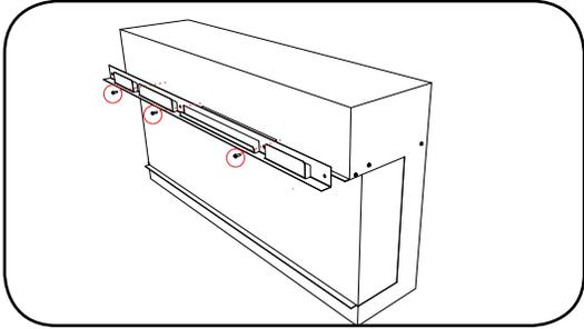
2. Remove existing side trim from unit by removing 3 screws in locations shown in Diagram below.
