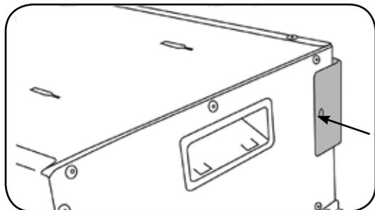
13. Fasten the two lower fixing bracket to the 2 fixing points on the underside of the appliance and secure to the wall, see Diagrams 18 & 19
