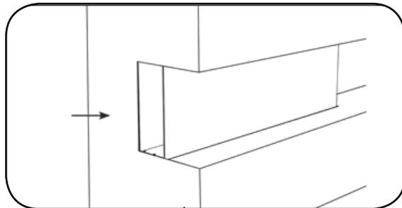
3. After the top and bottom installation have been completed, infills can be added to cover the dark areas of the side panels if desired, see Diagram below.
