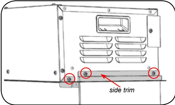
3. Install side mounting trim with four (4) screws in locations shown in Diagram below.
