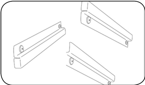
1. Support the bracket and remove the 3 screws, see Diagram below. Recycle bracket.
