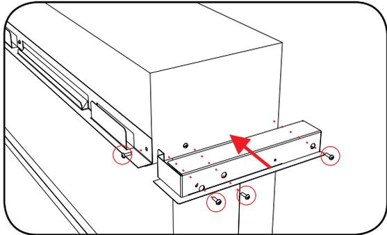
**Note:** There are holes in the side brackets to access the 3 screws on the side. Use a screwdriver long enough to reach these screws.
