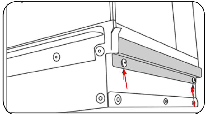
5. Fit the top Corner Side Glass Retainer bracket using 3 screws replaced in previous steps, see Diagram below.
