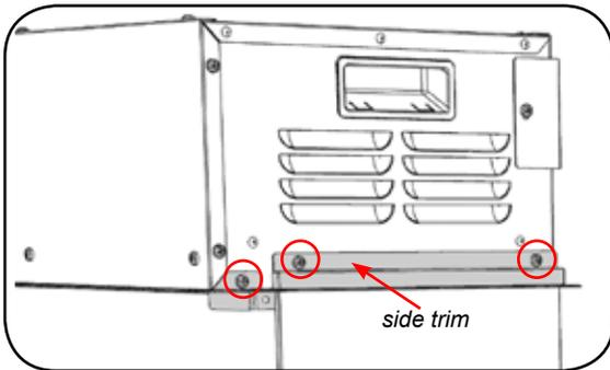
Note: Remove only the side trim which will be on the non finished wall side with the side glass exposed.
