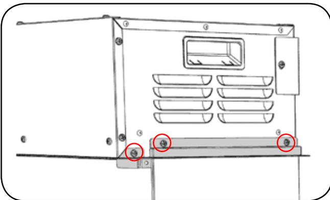
2. Remove the 2 screws securing the lower bracket, see Diagram below.
