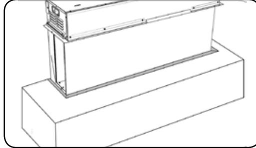
2. The lower enclosure can either create a floating shelf effect or a false chase box, see Diagram below.
