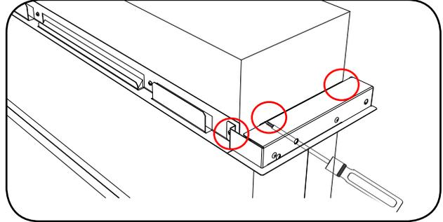
2. Remove existing side trim from unit by removing 3 screws in locations shown in Diagram below.
