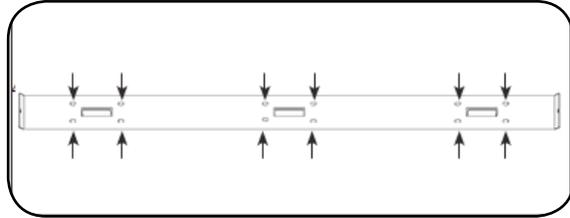
9. Drill the holes and insert the rawlplugs provided. Note: the rawlplugs supplied are suitable for solid wall application. If it is intended to mount the appliance onto drywall or hollow walls suitable fixing must be used.
