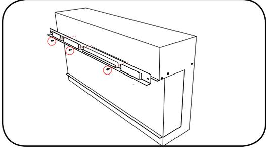
Note: There are holes in the side brackets to access the 2 screws on the side. Use a screwdriver long enough to reach these screws.
