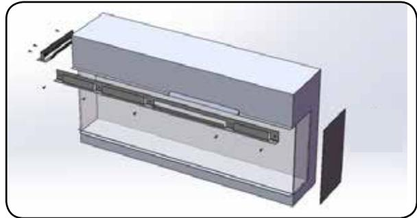
4. Fit the bottom Corner Side Glass Retainer bracket using both screws replaced in previous steps, see Diagram below.
