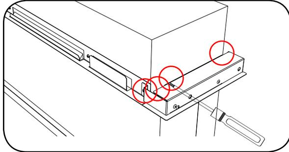
5. Install drywall directly onto mounting trims as shown in Diagram below.
