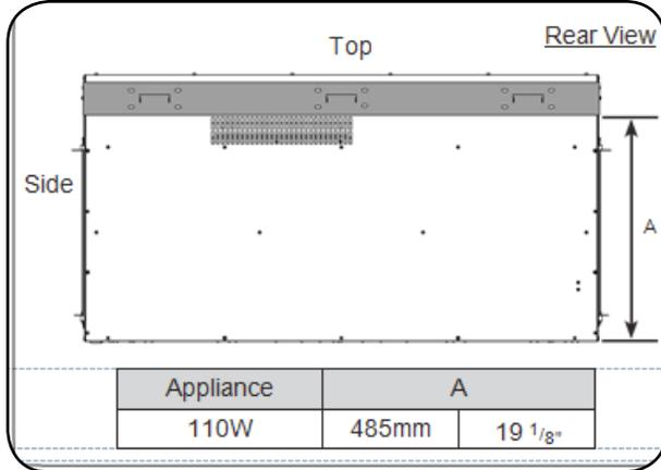
6. To prepare the installation measure the distance from floor level and using a spirit level draw a line A dimension higher than the intended position of the bottom of the appliance.
