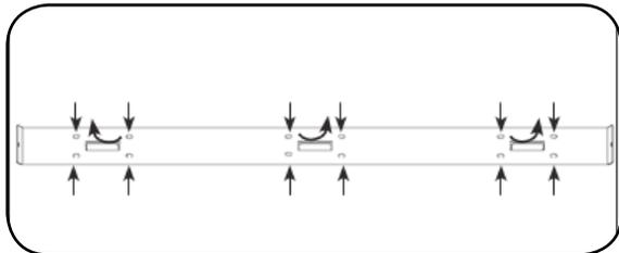
11. Lift the appliance onto the bracket. Ensure the folds locate into the slots on the back of the appliance, see Diagram below.
