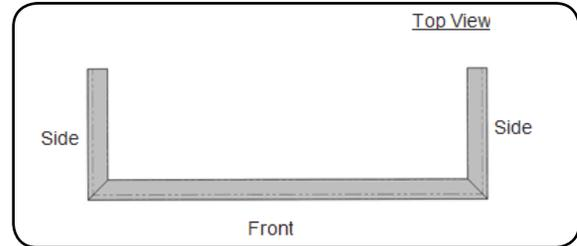
2. Place the decorative trims on top of the finished bottom enclosure, butt the trim up to the edge of the glass.
