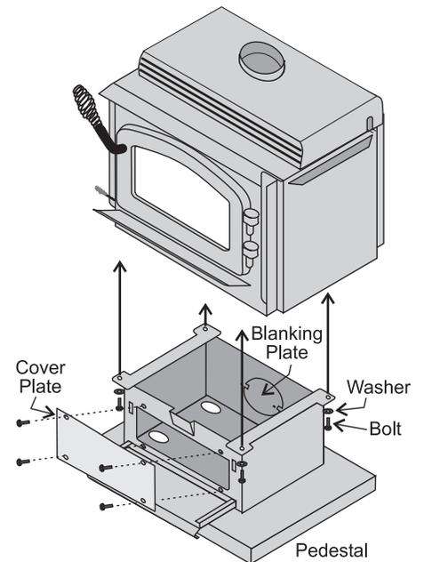
and must be installed unless the optional airmate has been selected. It stops the heat radiated from the flue collar from overheating the rear
