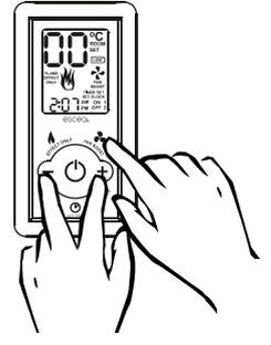
4. Press and hold the red auxiliary on/off button on the fireplace for a minimum of eight seconds, or until the two large temperature digits start counting upwards from 00 to 99 repeatedly.
